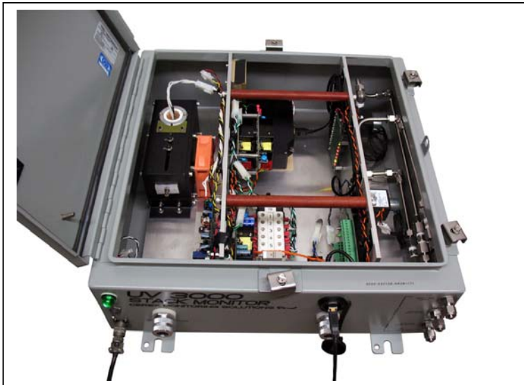
Cerex UV3000 Analyzer Internal View.
