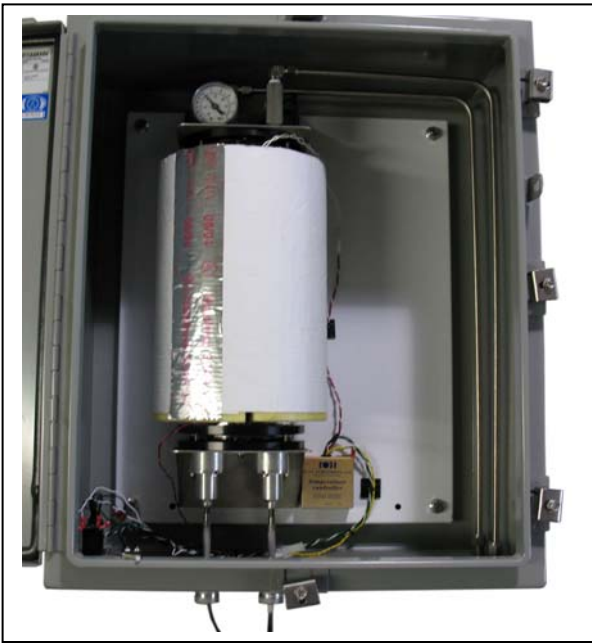
Cerex UV3000 Analyzer 10-Meter Multipass Cell Complete with Heating and Enclosure.
