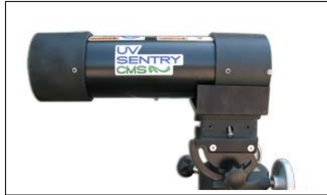
Shown above – The optical telescope “head” used in the cross-stack method of the UV3000 stack analyzer
