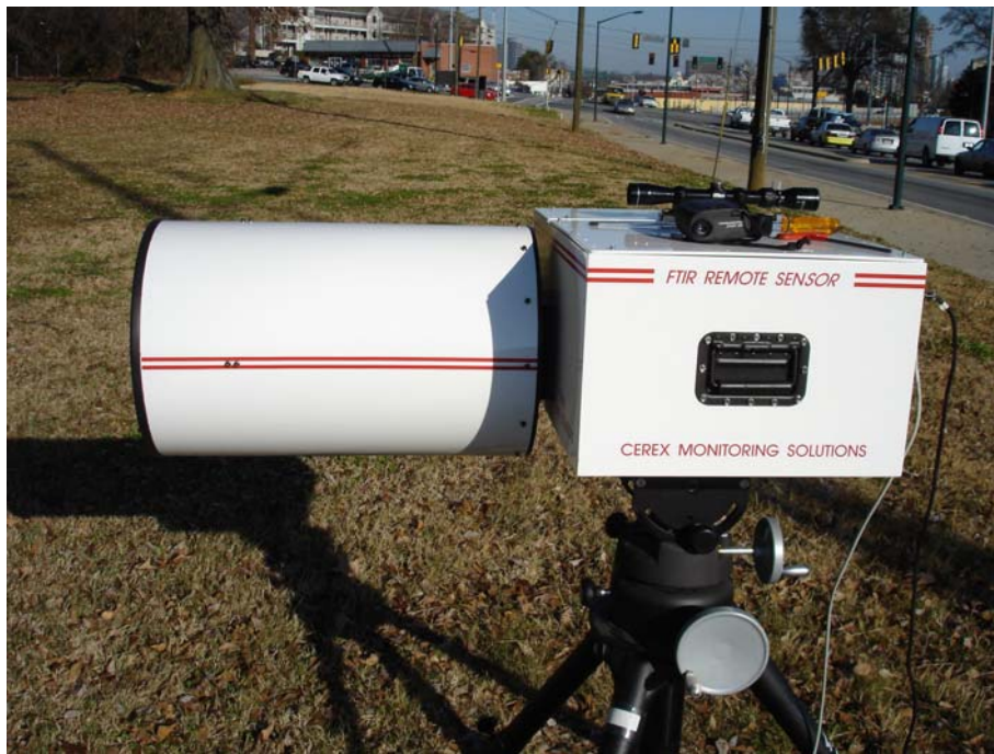
AirSentry under test outside the Cerex factory.
